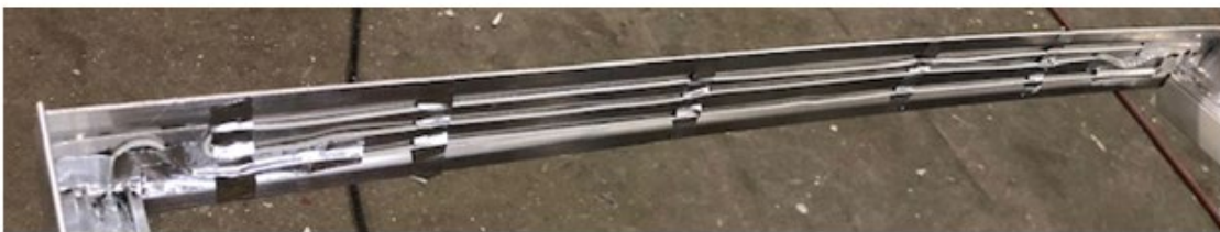
Picture 5.1. Heater wire routed all over the frame of the door, this picture shows the down step part of the frame.
