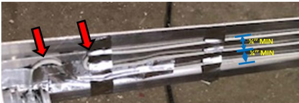
Picture 7.1. How to "snake" heater wire. Very important to keep space between routed wire \frac{1}{4} " apart as minimum and not allow any contact. |
